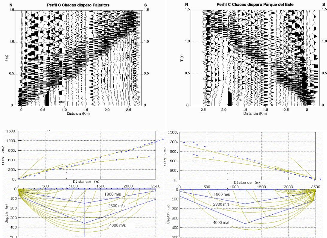
**Figure 6:** Seismic sections from the north-south profile crossing the Los Palos Grandes deep sedimentary basin (above) and preliminary 2D raytracing modelling (below) with observed (blue circles) and calculated (yellow lines) traveltimes.
