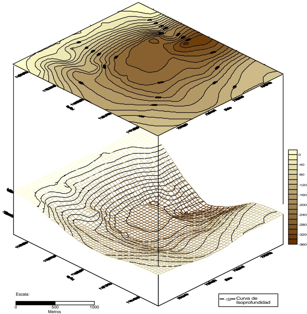
**Figure 4:** Contour map and isometry of sediment thickness in the Caracas valley derived from gravimetric modelling [11].
