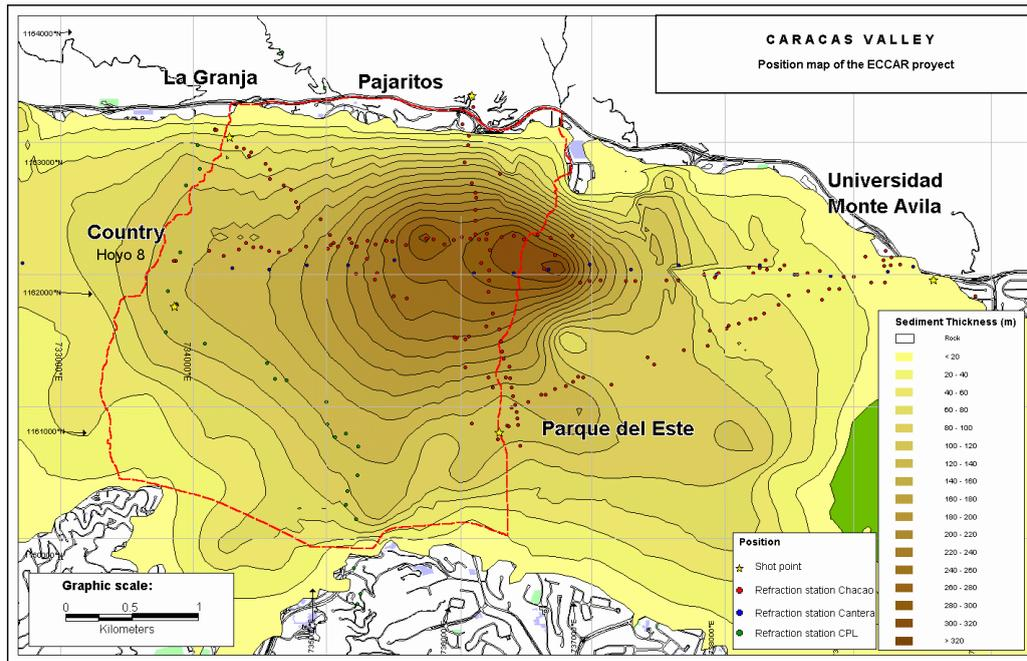
**Figure 5:** Map of sediment thickness [10] with the location of the seismic refraction profiles measured in July 2001 in the eastern part of the Caracas valley; for orientation see Figure 3.
